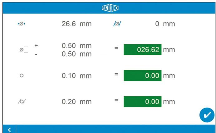
With the caliper, the forming results can be checked, including a freely selectable tolerance range. To do this, measure the workpiece at the point indicated by the red triangle.
