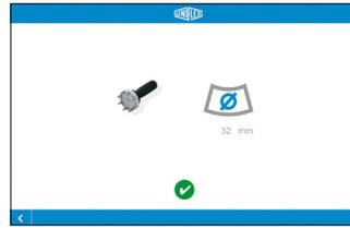
Input of crimping diameter, correction values and die set (automatic).
