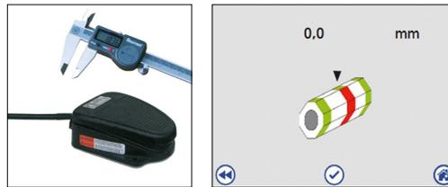
Measuring point menu with foot mouse/Vernier caliper (3 or 4"): Quality testing using calipers and foot mouse (as OK button). With the digital calipers, you can also check the crimping dimensions for conicity and ovality (number of measurement points). The pictogram-driven menu control guides you through the entire process.
