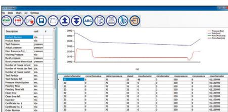
UTS enables a comfortable article entry via a PC. The data can be entered in a set MS Excel-sheet and be transferred with UTS to the Control C.2. Therefore, it is possible to compare the data from a number of machines, provide documentation and backup in one go. All crimpings can be documented with UTS, especially with the PFM option, which saves the pressure value as an additional parameter.
