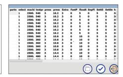
Displays the currently set log file overview. A log file may be selected and loaded to display or print it. The table lists all logs saved at the set storage location. All test-relevant data is shown. By scrolling to the right, other columns may be displayed. A log file is marked for opening by touching any cell in the line.
