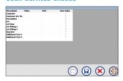
User-defined values may be created and saved for each item specifically and in any number. These values are not used by the control unit, but saved in the log file and may be printed in the record as well as shown and edited in the detail view. Examples for possible user-defined values are: Operator, Charge, Customer Item Number, etc.
