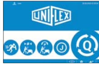
The queue mode sequentially executes individual pressing data sets stored in a database during production. This allows specific parameters to be determined and reported for individual workpieces (e.g., One-Piece flow).
