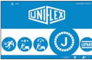
The job mode enables controlled processing of multiple orders in production. It is also possible to combine several orders from different data sets in the database into one work order. For this purpose, a quantity is assigned to each individual data set.
