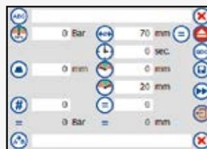
Input of pressure, hold time, opening diameter, preselection counter and press dies (parameter).
