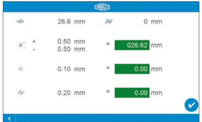
With the caliper, the result of the reshaping process can be checked using a freely selectable tolerance range. To do this, measure the workpiece at the position indicated by the red triangle.
