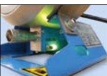
On SH 2 models, an optical signal is given when the crimp measure is reached. The electric and pneumatic variants have an automatic stop function.
