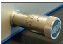
The micrometer allows you to set crimp dimensions to set. (Control A)
