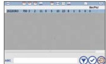
The user interface shows the database as a list of data records including names and test data. The requested data record is selected by a touch and is then highlighted blue.
