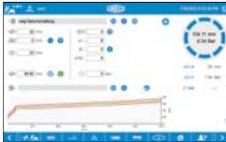
The PFM function enables continuous monitoring of the pressure or pressing diameter during production. If a parameter deviates from the learned target range, the pressing process is immediately stopped, and a message is displayed to the operator. This allows faulty components to be reliably detected during production.
