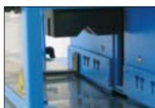
Exchangeable guide (two sizes) for optimum positioning of different hose sizes. (Only: EM 115)
