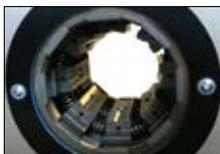
The large opening stroke allows you to pass 90° fittings without changing the crimp dies.
