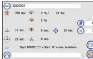
In the simple mode, an item can be uploaded from the database and the quantity can be selected; other settings cannot be made. The log file is recorded and, if selected, saved automatically.
