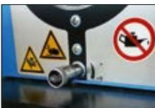
The micrometer allows you to easily set the crimping diameter.
