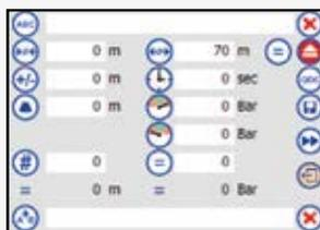
Input of press dimension, correction values, hold time, opening diameter, preselection counter and press dies (automatic).
