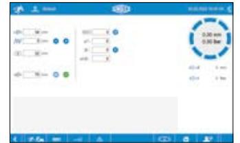
Input of press dimension, correction values, hold time, opening diameter, preselection counter and press dies (automatic).
