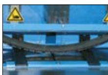
Various bending points selectable for straighter cuts and relief of pinch on the blad.
