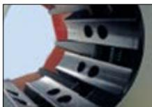
With the two-hole system, insertion of the dies from both sides is simplified and offers the possibility of selecting two different position (back and front) depending on the type of type of press jaw. The HM 3 H is compact and offers good accessibility.
