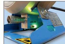
On SH 2 models, an optical signal is given when the crimp measure is reached. The electric and pneumatic variants have an automatic stop function.
