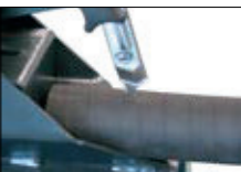
The SSG slitting tool shortens skiving chips up to 2".
