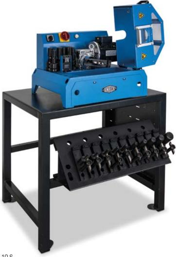
USM 10 S With TU Table and tooling storage (USM 10 S TU package).
