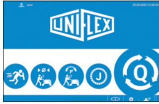
The queue mode executes individual press data records stored in a database one after the other during production managed from the server.
