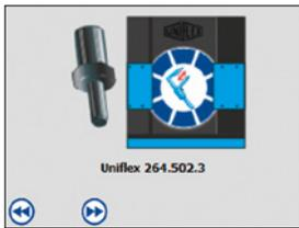
Calibrating your machine is simple using digital measurement via the software and the calibration mandrel.
