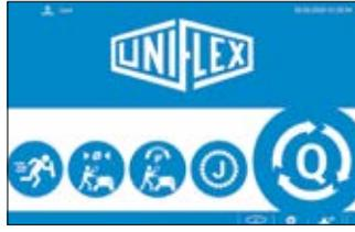
The queue mode sequentially executes individual pressing data sets stored in a database during production. This allows specific parameters to be determined and reported for individual workpieces (e.g., One-Piece flow).
