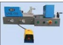
Preloading Safety control coupled to foot pedal.
