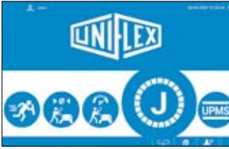
The job mode enables controlled processing of multiple orders in production. It is also possible to combine several orders from different data sets in the database into one work order. For this purpose, a quantity is assigned to each individual data set.
