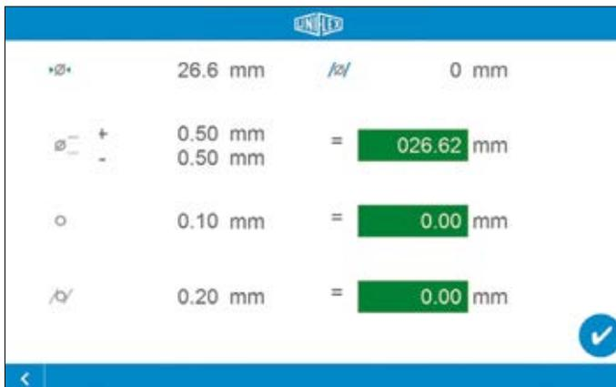
With the caliper, the result of the reshaping process can be checked using a freely selectable tolerance range. To do this, measure the workpiece at the position indicated by the red triangle.
