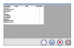
User-defined values may be created and saved for each item specifically and in any number. These values are not used by the control unit, but saved in the log file and may be printed in the record as well as shown and edited in the detail view. Examples for possible user-defined values are: Operator, Charge, Customer Item Number, etc.
