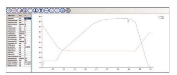
The UNIFLEX PFC (Pressure Force Control) option offers two ways to stop a compression – based on the distance travelled or the applied force, as happens with PFC. Stopping a compression stroke due to applied force can meet certain application requirements, specifically those where material behavior must be taken into account. This also makes it possible to press brittle materials, such as fibre glass. Many industry-leading glass insulator producers are already using PFC profitably.
