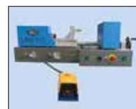
Preloading Safety control coupled to foot pedal.
