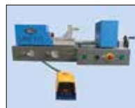
Preloading Safety control coupled to foot pedal.
