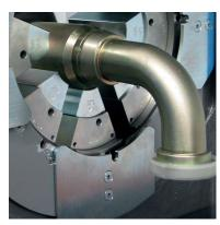
Due to our long master dies, you can crimp virtually all types of fittings. This slide bearing technology reduces friction by 20% and ensures high process stability and
