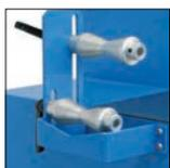
Lateral guide rolls for guiding and positioning of the hose, for a better cutting quality.
