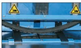
Various bending points selectable for straighter cuts and relief of pinch on the blade.
