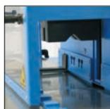
Exchangeable guide (two sizes) for optimum positioning of different hose sizes. (EM 115 only)
