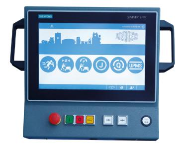
Industrial PC with 12" touch panel integrated RFID reader
