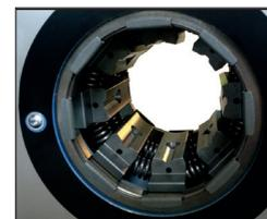
The large opening stroke allows you to pass 90° fittings without changing the crimp dies.
