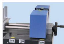
Axially adjustable clamping unit - prevents bending of small hose dimensions.
