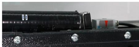
UNIFLEX insert – marking tool (ferrule position marking increases productivity and improves safety in hose sizes up to 2").
