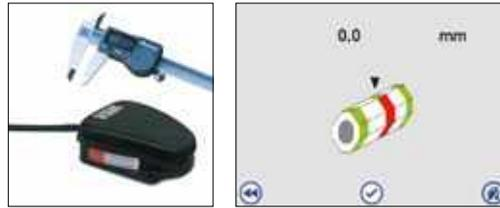
Measuring point menu with foot mouse/Vernier caliper (3 or 4"): Quality testing using calipers and foot mouse (as OK button). With the digital calipers, you can also check the crimping dimensions for conicity and ovality (number of measurement points). The pictogram-driven menu control guides you through the entire process.
