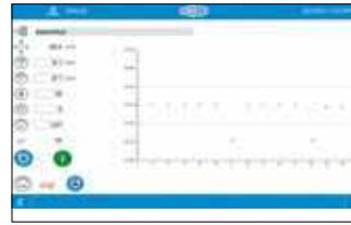
The machine capability index (CMK) describes the ability of the machine to meet the specified requirements. With the CMK function in the control, it is possible to set the characteristic values of the machine capability.
