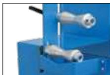
Lateral guide rolls for guiding and positioning of the hose, for a better cutting quality (EM 115)
