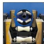
Clamping and guiding unit with wheels for up to 5"-hoses.
