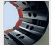
With our two position holes-system, the insertion of all dies from both sides is easy and quick. You can also choose two different options to position your die set.
