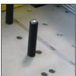
Guide pins ensure straight cuts, which prolongs EM 1 EM 2 blade life.
