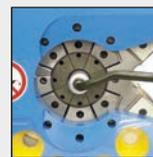
Radial insertion of workpieces, catering even to 90° bends.
