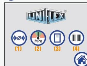
Four choices for selecting compression parameters quickly and easily. Selection menu includes pressing by dimension, by pressure, stored parameters in integrated database in the controller, or by use of a barcode scanner.
