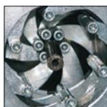
Improved fixture for centering hose clamp. Longer, grooved rollers ensure a better grip.
