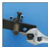
Blade adjustments for skiving depth need only to be made once for each hose dimension on the USM 10 S.
