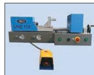
Preloading Safety control coupled to foot pedal.
