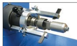
Simultaneous internal and external skiving. (USM 100)
