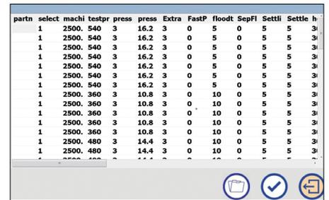
Displays the currently set log file overview. A log file may be selected and loaded to display or print it. The table lists all logs saved at the set storage location. All test-relevant data is shown. By scrolling to the right, other columns may be displayed. A log file is marked for opening by touching any cell in the line.
